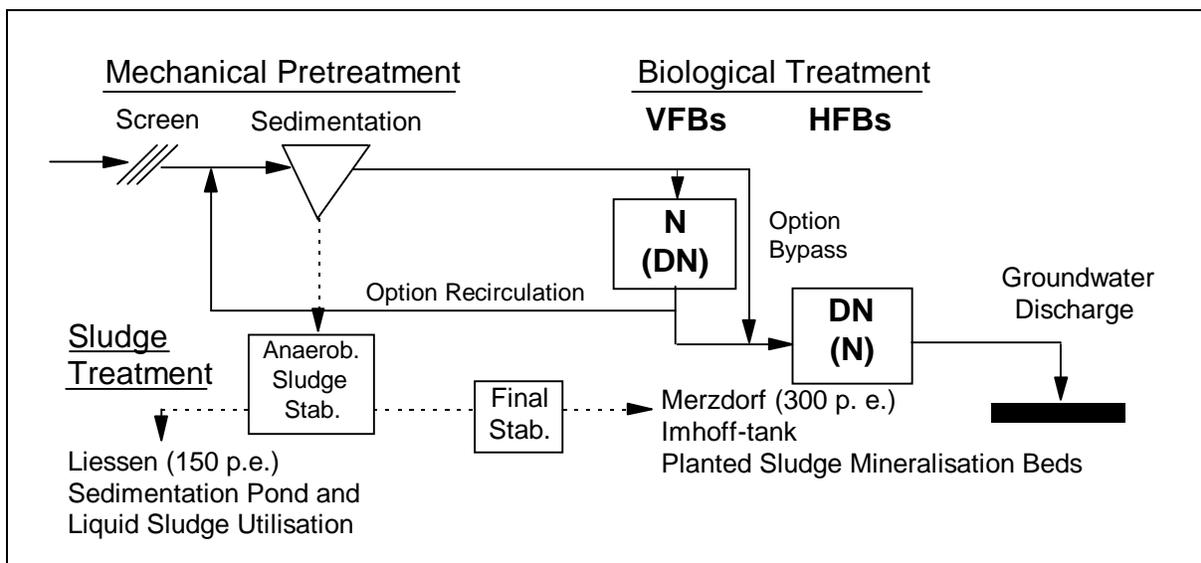
Figure 1:Flow scheme of a combined system treatment plant
