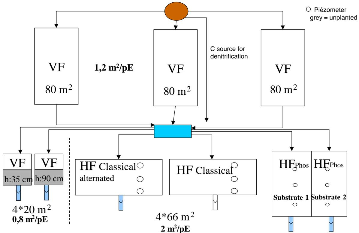
Figure 2 Flowsheet of the hybrid system proposed for Evieue (Boutin et al., 2000)
